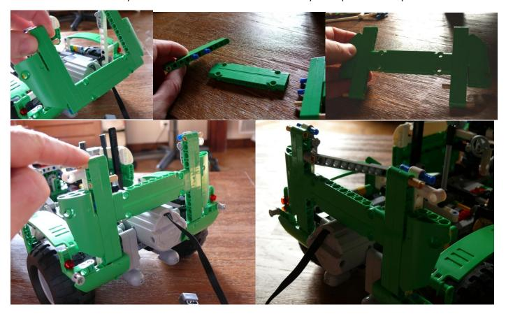
Now, let's proceed with the servormotor used for steering. Assemble the following pieces
